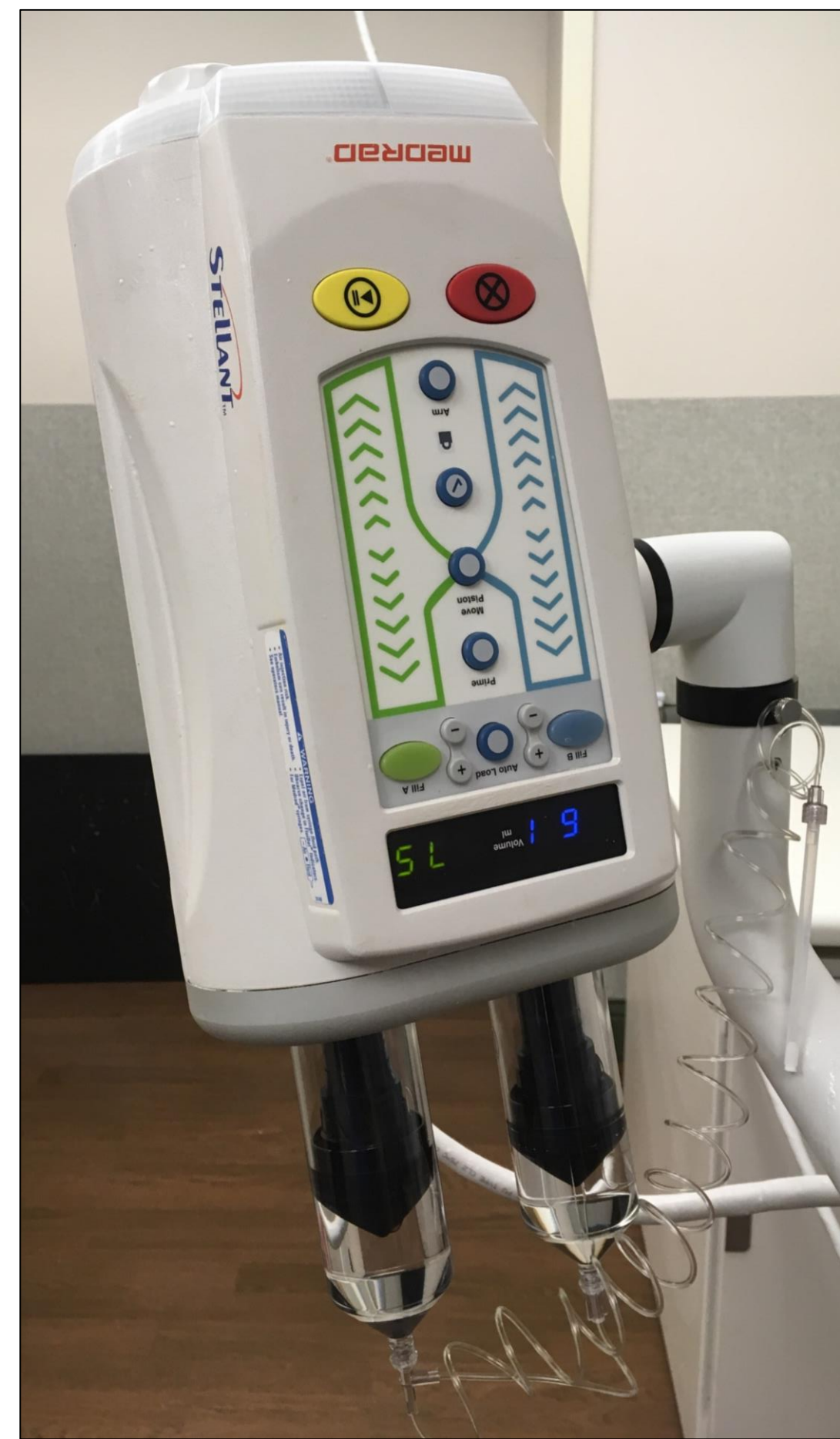
Figure 1: MedRad Stellant Dual Syringe injector injecting a small volume of saline (blue column) at the same rate as the IV contrast (green column) prior to contrast injection.
