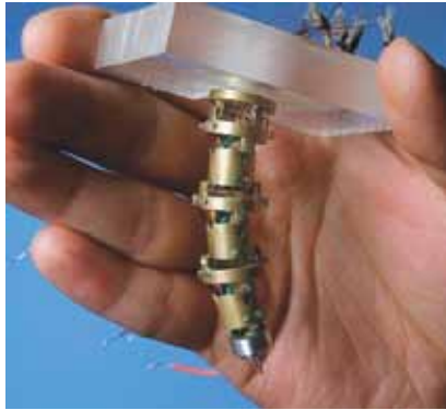
The newest prototype of the MR imaging-compatible Minimally Invasive Neurosurgical Intracranial Robot (MINIR) ( above ) designed to enable neurosurgeons to reach and remove brain tumors and greatly improve patient outcomes; ( bottom right ) an earlier version of the MINIR; Jaydev Desai, Ph.D., ( bottom left ) is among the University of Maryland School of Medicine researchers who developed the MINIR prototype.
