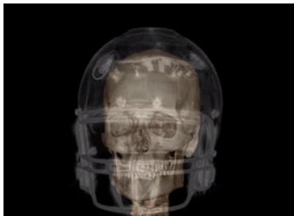
Video 1. Animation showing how the HIT system accelerometers fit around the player's head. The springs ensure the sensors remain in contact with the head, measuring head acceleration not helmet acceleration.
