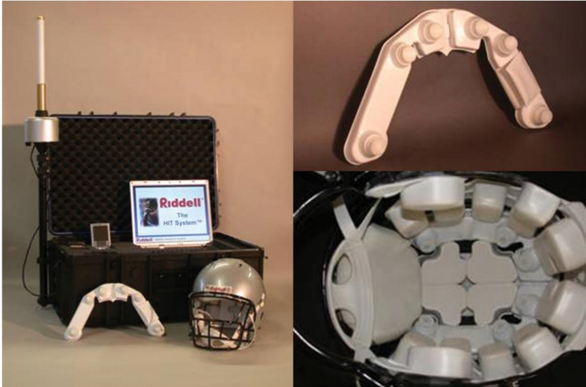
**Figure 3.** Riddell HIT System with a sensor array and helmet.
