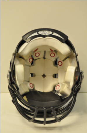
Figure 2. Helmet with embedded sensors
