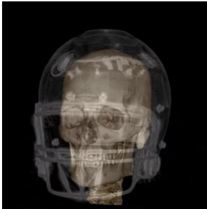
Video 1. Animation showing how the HIT system accelerometers fit around the player's head. The springs ensure the sensors remain in contact with the head, measuring head acceleration not helmet acceleration.
