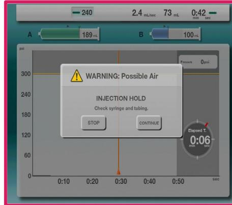
b) When the injector recognizes the air and stops it
