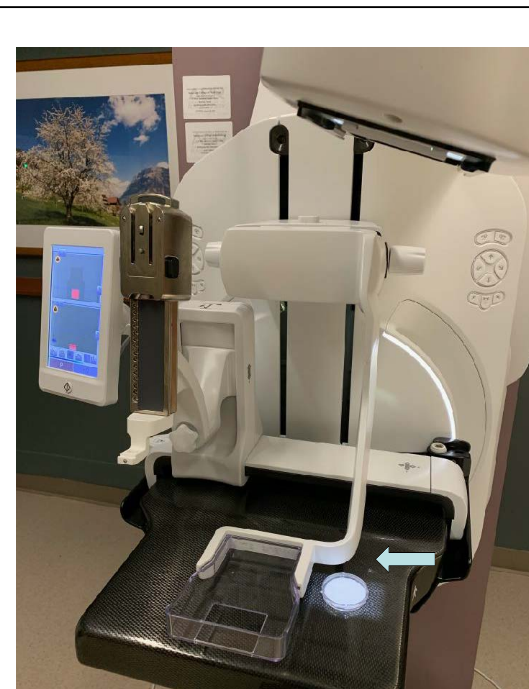
Fig. 1- A photograph of a pre-procedure set-up of a mammography unit demonstrating a biopsy attachment with a fenestrated compression paddle (Serena Bright™, GE Healthcare, Buc, France), as well as a round plastic specimen container within a rectangle of light for specimen radiography in the right upper corner of the mammography plate (arrow). Specimen radiography can be done on either side of the compression paddle depending on the breast and needle position.
