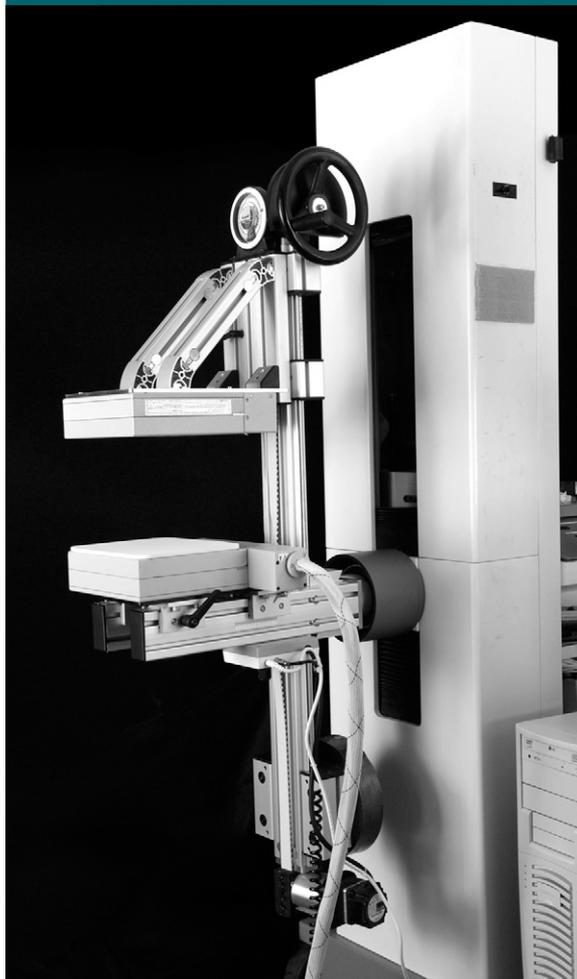
**Figure 1:** Dedicated dual-head gamma imaging system comprising two CZT-based gamma cameras mounted on a modified mammographic gantry. The breast is positioned between the two detector heads and lightly compressed.
