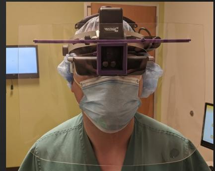
3D printed face shield for Keeler Indirect Ophthalmoscope
