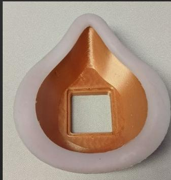
Masks were fitted with a platinum silicone gasket, which rests directly against the face, adhered with silicon adhesives. The gasket design both improves comfort for the mask wearer and allows for an airtight seal.
