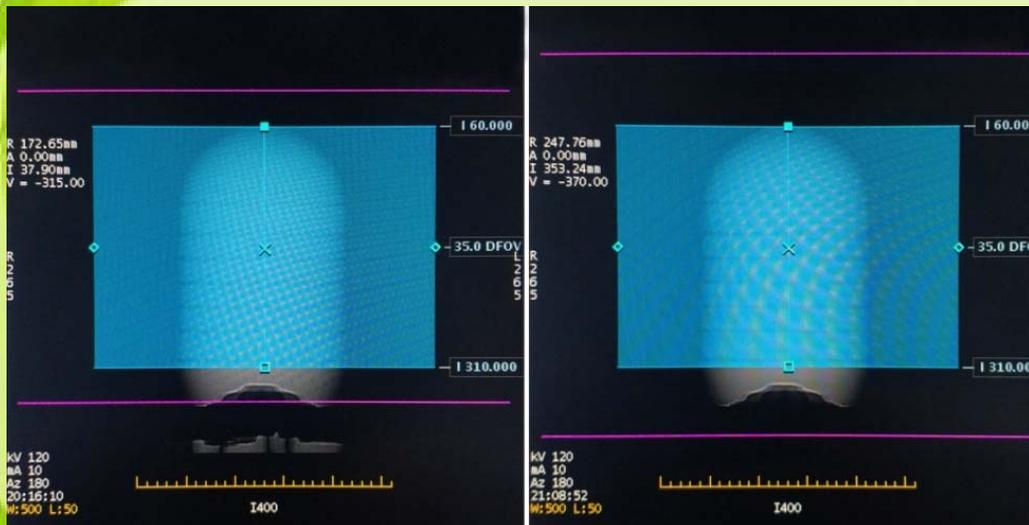
**Picture 1** The z over-scan of 40mm (left , about 3cm in one side) and 80mm detector coverage(right , about 6.2cm in one side).
