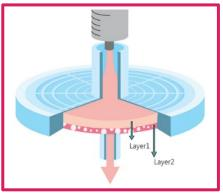
b) Syringe filter illustration to which the same principle is applied https://www.ud-technology.com/syringe-filter
