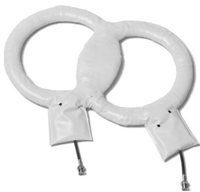
Figure 1: Custom-built quadrature RF transmit-receive surface coil consisting of two 13-cm elements used for our study at 7 T.
