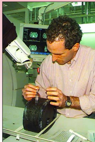
Dr. Wood is validating on a phantom the exquisite accuracy of the CT robot for "point and click" needle insertion and tumor destruction. Courtesy Philips Medical Systems
