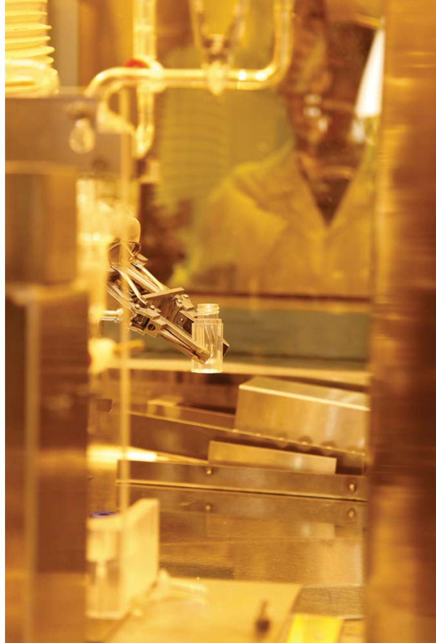
The inside view of a medical isotope hot cell.
